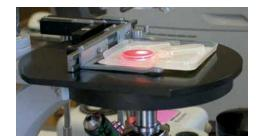
Place the unopened InTray on the stage with Place the unopened InTray on the stage with the yellow label facing up.
